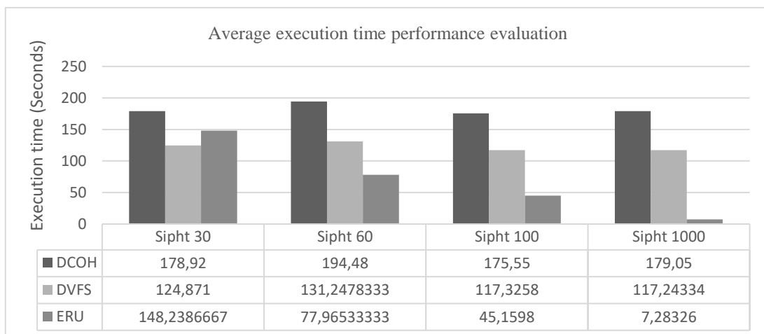
Figure 5. Average execution time comparison using proposed ERU model with multi-objective based DVFS-based workload scheduling algorithm
